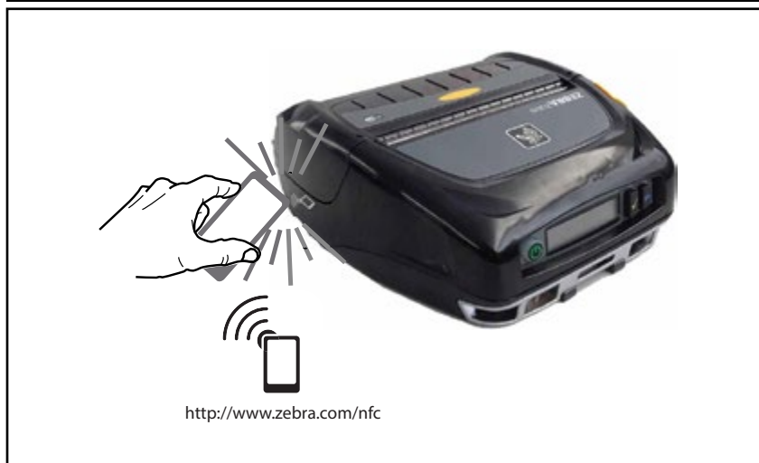
Figure 14: Near Field Communication (NFC) Pairing
