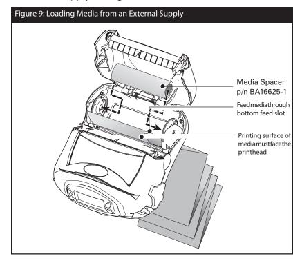
dia guides and up through the media compartment as shown. Make sure the side of the media you will be printing on faces the printhead.
