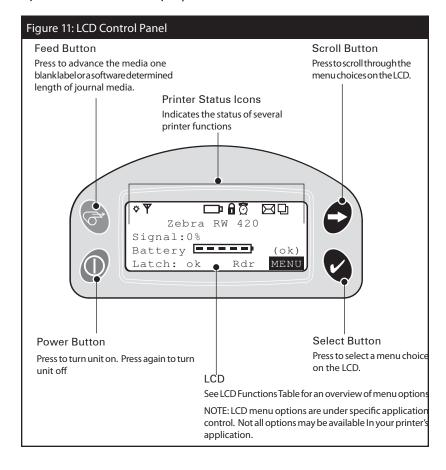
The top of the screen has a row of status icons which indicate the state of various printer functions:
