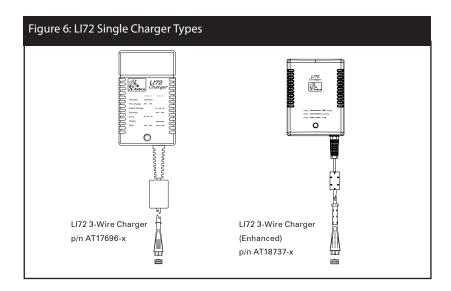
Two three-wire versions of the LI72 are offered as illustrated in Figure 4. The enhanced 3-Wire version (AT18737-x) offers improved charging features and will replace the LI72 3-Wire charger (AT17696-x).
