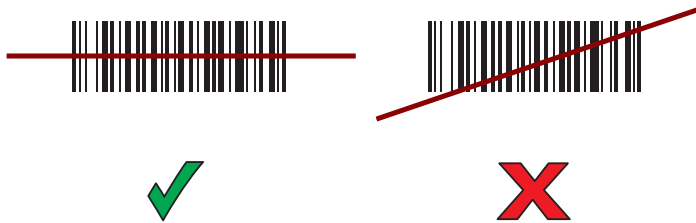
Figure 40 Laser Scanner Aiming Pattern
