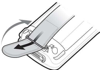
**Figure 1-18** *Slide Handstrap through Clip*
