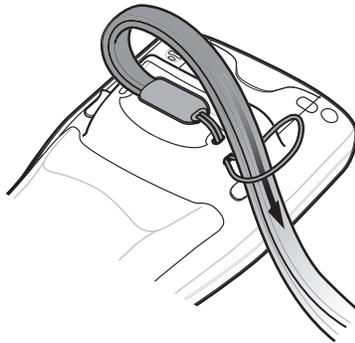
**Figure 1-13** *Slip Wrist Strap Through Loop*
