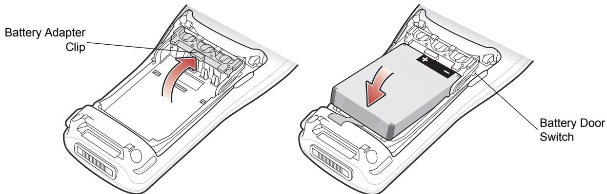
**Figure 1-3** Battery Insertion
