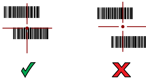
Figure 17 RS6000 Pick List Mode with Multiple Barcodes in Aiming Pattern
