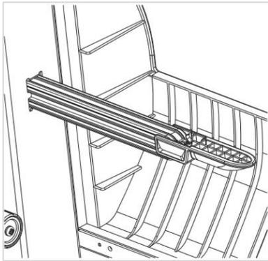
1. Move the label roll guard horizontally to the end of label spindle, then flip down the label roll guard.
