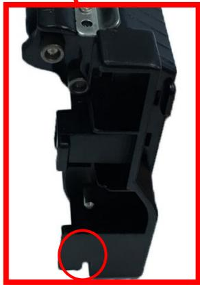
6. After the connection is completed, groove foot on the peeler to the base iron plate near the panel, and then gently push it to the left.
