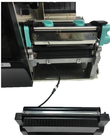
5. After pulling out the wafer 1x3P P2.0 of the printer, connect it to the wafer 1x3P P2.0 of the peeler.
