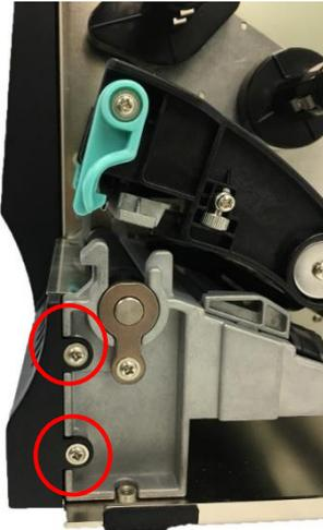
2. Remove the two screws located on the side of the cover.
