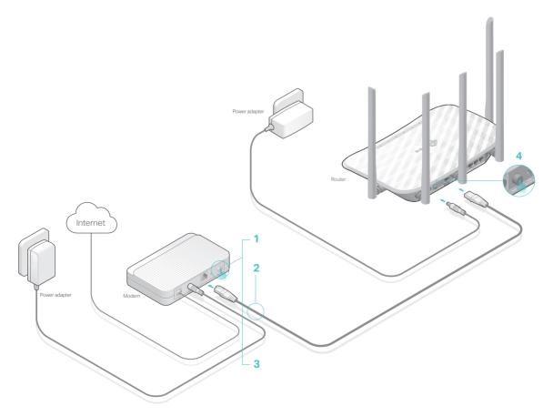
1. Turn off the modem, and remove the backup battery if it has one.
