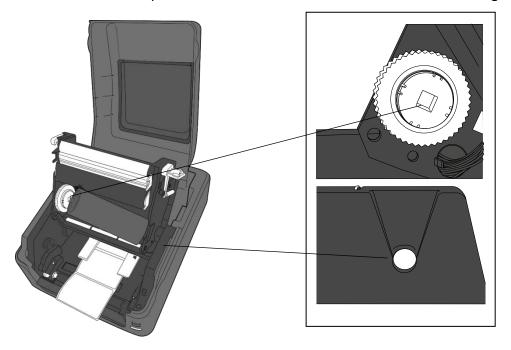
• To load the take-up roll, set the empty ribbon core on the core adapter
