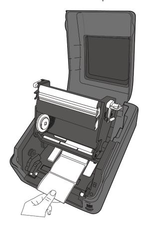
Put the media under the Media Shaft and center it between the Media Guides.
