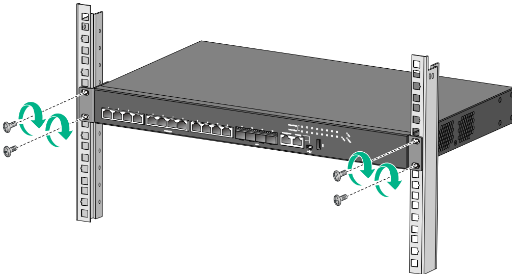
Figure 5 Mounting the switch in the rack (front mounting brackets at the port side)
