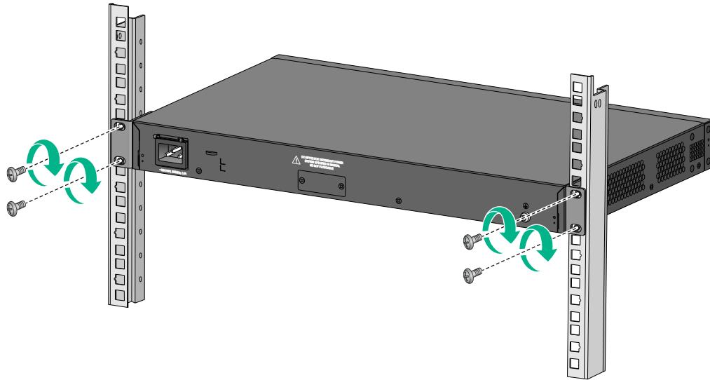
Figure 6 Mounting the switch in the rack (front mounting brackets at the power module side)
