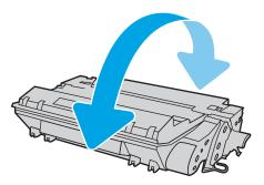
7. Align the toner cartridge with the tracks inside the printer, and install the toner cartridge until it is firmly seated.
