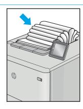
The paper does not stack well in the output tray. The stack might be uneven, skewed, or the pages might be pushed out of the tray and onto the floor. Any of the following conditions can cause this defect:
