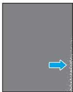
Toner rubs off along either edge of the page. This defect is more common at the edges of high-coverage jobs, and on light media types, but can occur anywhere on the page.
