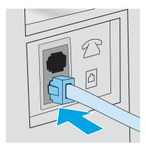
4. Connect the answering machine telephone cable to the telephone line out port on the rear of the printer.
