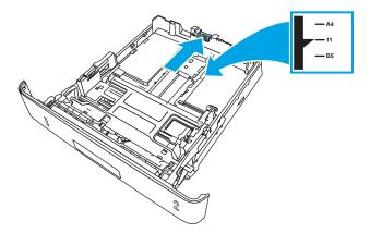
4. Load the paper into the tray. Make sure that the stack is flat at all four corners and that the top of the stack is below the maximum-height indicators.
