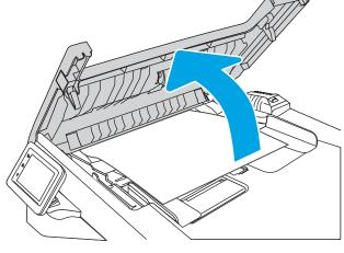
2. Use a moist, lint-free cloth to wipe both pickup rollers and the separation pad to remove dirt.
