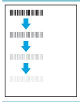
Slight shadows or offsets of the image are repeated down the page. The repeated image might fade with each recurrence.
