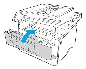
8. If no paper was jammed inside the print cartridge door, press the front door release button.
