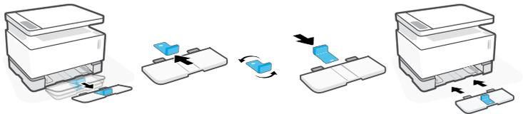
1. Tilt up the input tray slightly and pull it off the printer.
