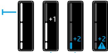
**Fill:** Toner is partly depleted. "+1" means one HP Toner Reload Kit can be added.
