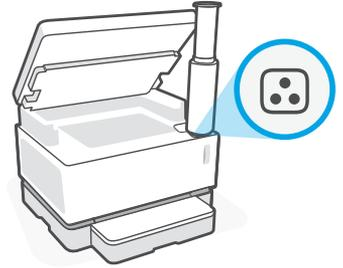
Toner can be added when the **Reload Status** light (Ⓜ) next to the reload port glows white. Toner cannot be added when the light is off. To learn how to add toner, follow the instructions on the HP Toner Reload Kit or download the User Guide from [www.hp.com/support/Neverstop1200](http://www.hp.com/support/Neverstop1200).
