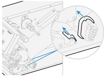
13. Route the media through the cutter between the two guide plates.
