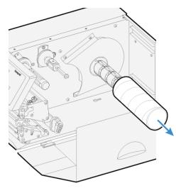
6. If your are using a media roll with a 76 mm (3 in) core, fit an adapter on the media supply hub.
