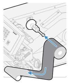
7. Without releasing the ribbon, turn the printhead lift lever clockwise to lower the printhead and lock the ribbon.
