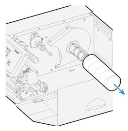
6. If you are using a media roll with a 76 mm (3 in) core, install a 3-inch adapter on the media supply hub.
