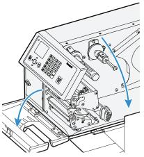
2. Pull the upper guide straight out and press the snap-lock, lift the edge of the lower guide, and pull the lower guide straight out.
