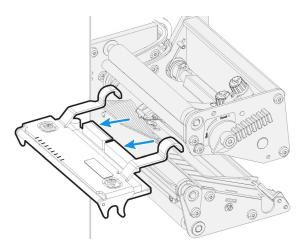
9. Connect the two cables to the replacement printhead.
