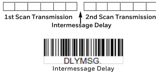
To remove this delay, scan the Intermesage Delay barcode, then set the number of delays to 0. Scan the Save barcode from the [Programming Chart](#), beginning on page 211.
