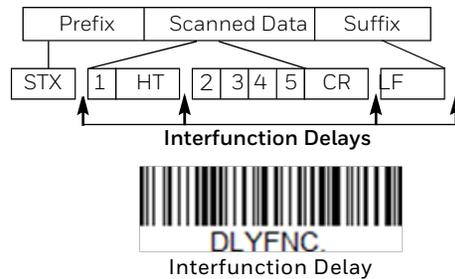
To remove this delay, scan the Interfunction Delay barcode, then set the number of delays to 0. Scan the Save barcode from the [Programming Chart](#), beginning on page 211.
