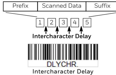
To remove this delay, scan the Intercharacter Delay barcode, then set the number of delays to 0. Scan the Save barcode from the [Programming Chart](#), beginning on page 211.
