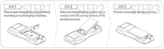
\* When the cover is not closed correctly the portable terminal will not be turned ON.
