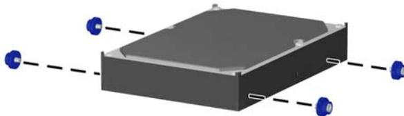
8. Align the guide screws with the slots on the chassis drive cage, press the hard drive down into the bay, then slide it back until it stops and locks in place.
