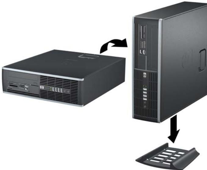
📝 **NOTE:** To stabilize the computer in a tower orientation, HP recommends the use of the optional tower stand.
