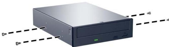
5. Slide the drive into the drive bay, making sure to align the guide screws with the guide slots, until the drive snaps into place.
