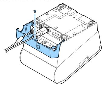
• To remove the connector cover, turn the printer over, remove the screw, and push the connector cover down while pushing both sides of the connector cover inward to detach the hooks from the printer case.
