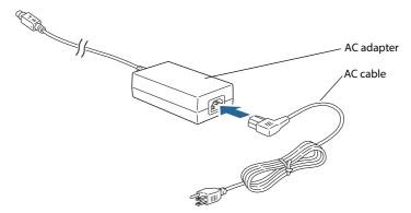
Connect the DC cable of the AC adapter to the power supply connector (stamped 24V).
