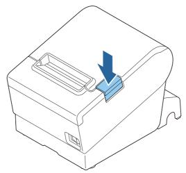
Install the roll paper guide so that the protrusion on the roll paper holder is aligned with the hole on the printer.
