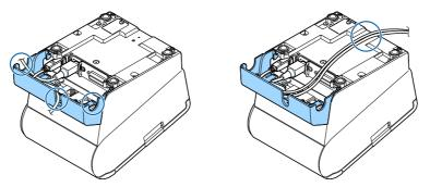
If you want to pass the USB cable through the cable exit on the back, fit the cable under the hook on the printer to prevent the cable from coming off and to prevent too much force being applied to the connector section.
