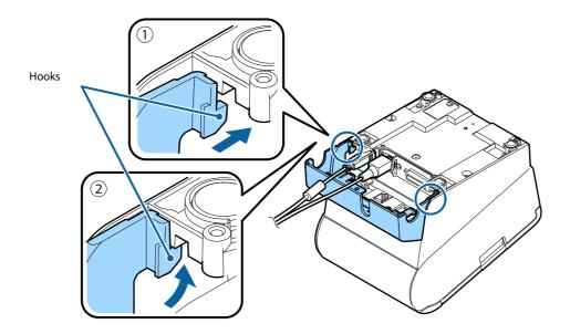
**?** Push the connector cover down to click onto the printer case.
