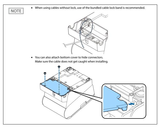
After the cable arrangement, turn over the printer, and make sure the cables are not pinched.
