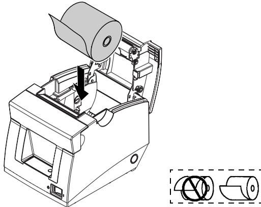
4. Pull out some roll paper as shown in the illustration below, and close the printer cover.
