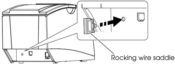
2. Hook the USB cable with the locking wire saddle.
