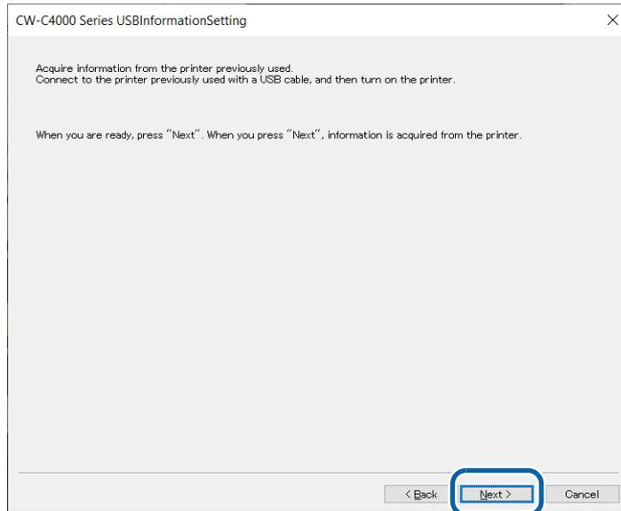
**4** Information of the old printer is acquired. Then, disconnect the old printer from the computer.
