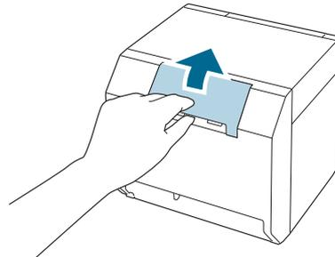
**4** Remove the paper feed guide, and then close the rear cover.
