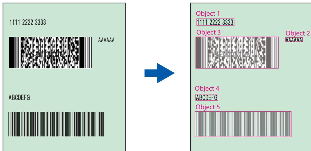
Example when scaled down by 1.5% both vertically and horizontally with the positioning functions
