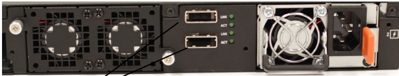
Figure 3-13. N3048 Mini-SAS Stacking Ports Close-up
