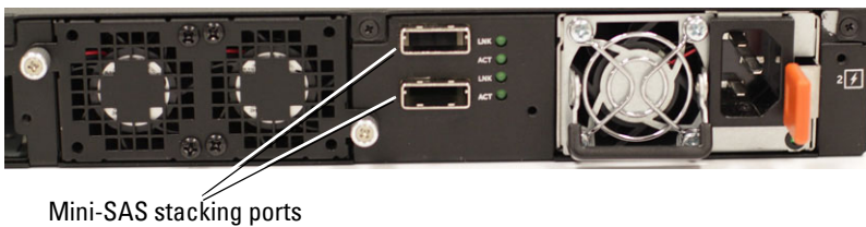
Figure 3-22. Dell EMC Networking N3048 Mini-SAS Stacking Ports Close-up
