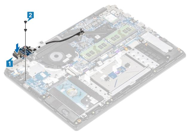
Route the VGA board cable through the routing guides on the fan [1], and then connect the VGA daughterboard cable to the system board [2].
