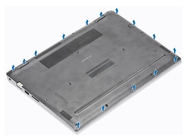
3 Lift the right side of the base cover [1], and remove it off the palmrest and keyboard assembly [2].
