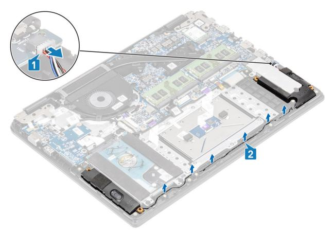
3 Lift the speakers, along with the cable, off the palm rest and keyboard assembly.
