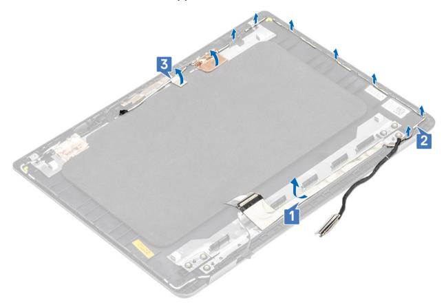
3 Lift the camera cable and the display cable off the display back-cover.
