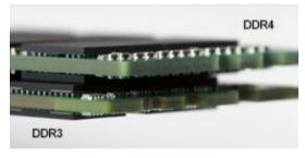
Figure 2. Thickness difference
