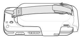
9. Place hand between device and hand strap and adjust hand strap as necessary.
