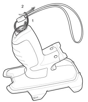
3. Pull the lanyard until the loop tightens.
