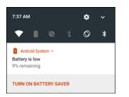
When the battery charge drops below 10%, the TC20 displays a notice to connect the TC20 to power. The user must charge the battery using one of the charging accessories.
