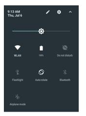
2. Touch WLAN to open the WLAN screen. The TC20 searches for WLANs in the area and lists them.
