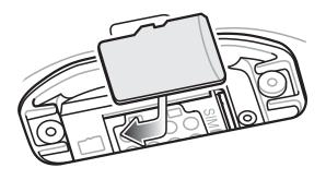
10. Push the microSD card into the SD card slot.
