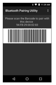
4. Using the RS507/RS6000, scan the barcode on the screen.
