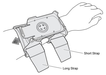
3. Tighten both straps on forearm and press hook and loop material together.
