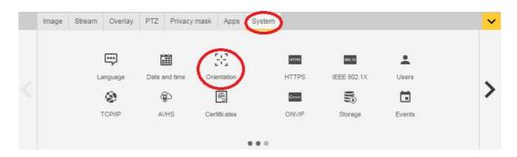
After the setup is completed, it is still possible to change the configurations in the camera's web pages. To change the dewarped view or perspective mode, go to **System > Orientation**.
