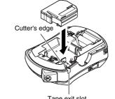
Make sure that the end of the tape feeds under the tape guides · Use only Brother M tapes with this machine. Attach the back cover by inserting two
