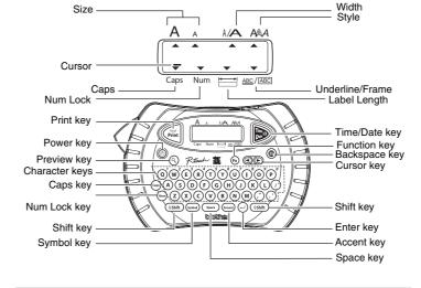
The LCD shows one row of 8 characters; however, the text that you enter can be up to 80 characters in length, which will scroll across · Use Cursor key while holding down Shift key to go to beginning /
