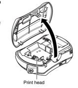
Insert four new AAA-size alkaline batteries (LR03), making sure that their poles point in the correct directions. Always replace all four batteries at the same time using brand
