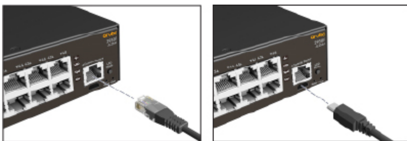
Figure 21: Connecting a console cable
