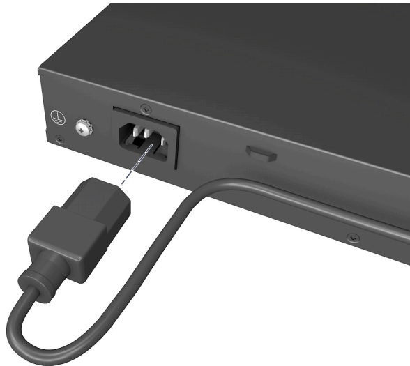
Figure 18: Connecting the power cord on 2930F 24-port and 48-port switches
