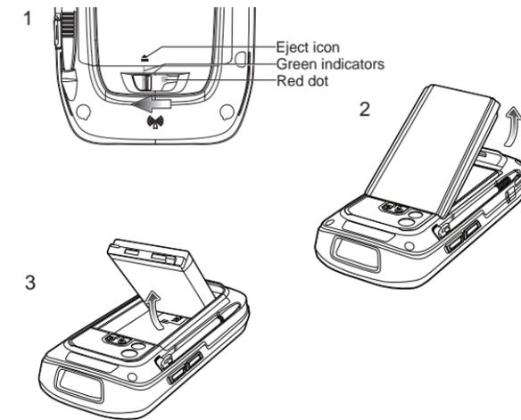
Note: To unlock and remove the battery cover, slide the battery cover latch to the left until the green indicators align with the eject icon and the red dot is visible. The battery cover ejects slightly. Lift to remove.
