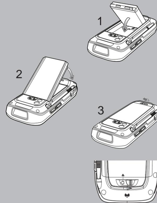
Note: To lock the battery cover, slide the battery cover latch to the right until the red dot is not visible.
