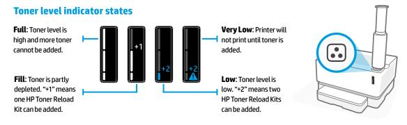
Toner can be added when the **Reload Status** light . next to the reload port glows white. Toner cannot be added when the light is off. To learn how to add toner, follow the instructions on the HP Toner Reload Kit or download the User Guide from www.hp.com/support/Neverstop1000.
